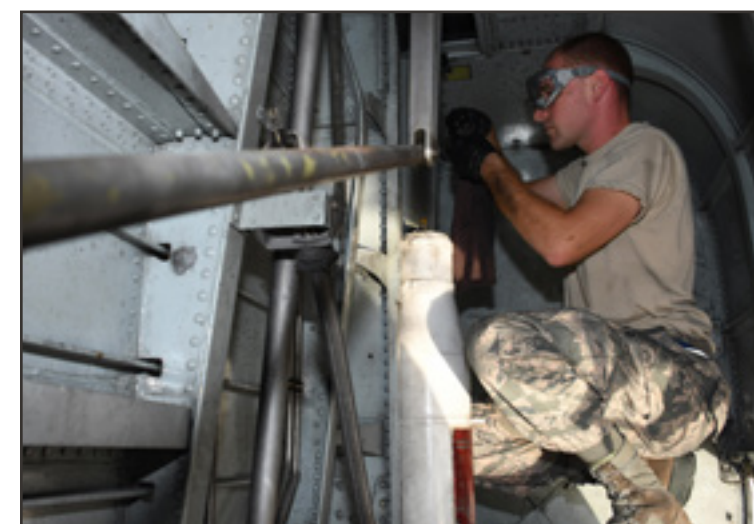
Staff Sgt. James Swann, a crew chief, applies lubricant to the landing gear of a C-130 Hercules at Al Udeid Air Base, Qatar, Dec. 30, 2016.
